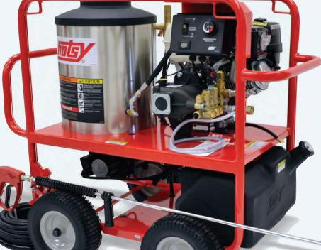
**Control box** with adjustable temperature control lighted burner On/Off switch and hour meter
